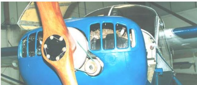
Birds also find aircraft irresistible nesting sites; a nest removed in the morning may be substantially rebuilt by late afternoon. Pre-flight checking the aeroplane becomes very important. Insects may take over your aircraft. Given a few days undisturbed progress, a wasps' nest could appear.
