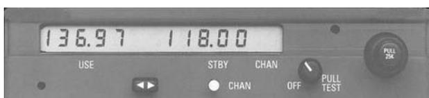
b) GA aircraft VHF radio equipment typically has 760 channels spaced at 25 kHz; some older radios have only 720 channels with an upper limit of 135.975 MHz, these are not allowed for IFR flight, or for VFR flight in certain countries including Germany.
